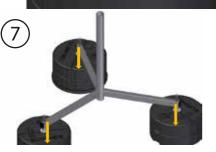
Repeat previous steps for each assembly element in the set, afterwords insert a tripod frame the way its shown on a drawing.
