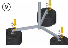
Apply and tight the nut M16 and second regulation nut M16, to all assembly elements.
