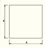
For mechanical damage protection of roof surface. To use under concrete base of mast. Depending on roof covering type use appropriate pad: tar board or membrane.
