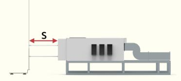
Keeping the insulation clearance using insulated high-voltage cable system — used in places where it is not possible to keep the insulation clearance due to the lack of space on the roof or the architectural point of view to keep aesthetics of the facility. High-voltage cable system compliant with the PN-EN 62305 standard provides us with an insulation clearance of 75 cm.
