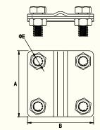
For cross wire connections. Two parts 2 mm thick, assembled with 4 screws M8. Option 90100101 suitable to connect wires up to Ø 8mm, as option 90100201 suitable to connect wires up to ø 10mm.
