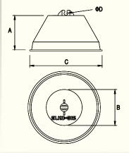
For fixing wire on the flash roofs. Can be glued to roof surface using glueing composition 99401099 (only option with concrete bottom). Glue assembly details, see: <a href="https://www.elkobis.com.pl/download">www.elkobis.com.pl/download</a>.
