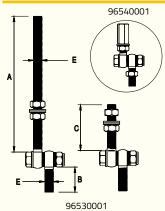
For vertical-lining of masts including roof slope. It is recommended to use regulation sets above 3% slope. Set 96530001 dedicated to vertical-lining of tripod masts up to 25% roof slope.
