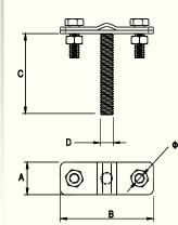
For insulated bars wire conductors leading. Insulated bars should be firstly mounted to steel construction, device cover or interception air rods.
