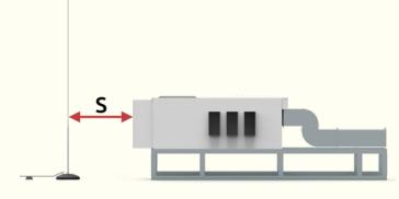
Maintaining the insulation clearance on insulation bars - used in places where mounting to the device or shutter structure is possible. By using insulation bars made of non-conductive material, we keep the insulation clearance despite mechanical connection
